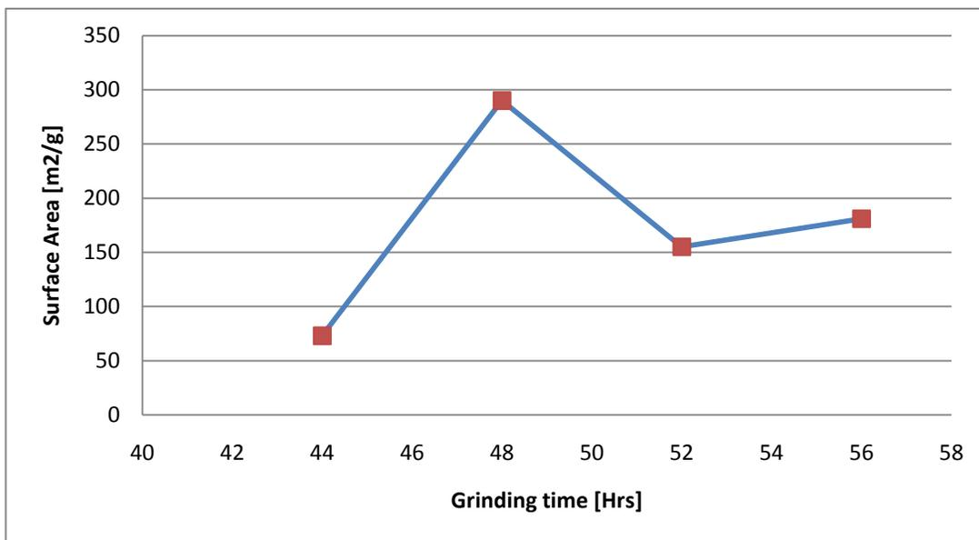
It can be clearly seen that, for this particular SiC material, milling beyond 48 hours is, as a result of overgrinding, counter-productive.
